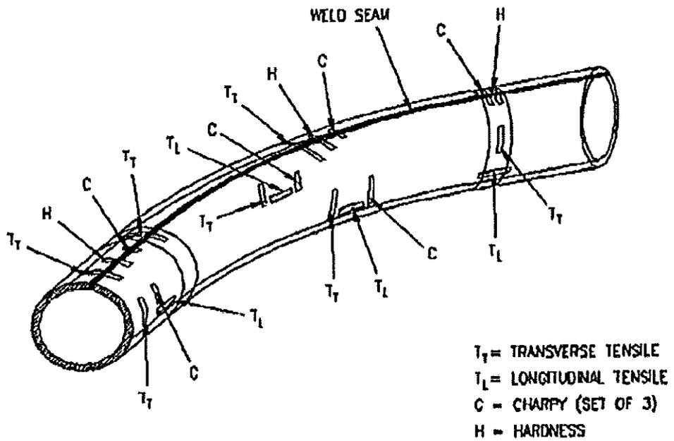
Figure 3.1 Mechanical Testing of Induction Bonds
